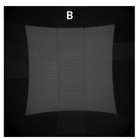
Dot projector **'B**' has a FOI of 70° x 70° and like design 'C' demonstrates a record efficiency above 70% even with its comparably larger FOI.
