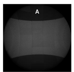
Dot projector '**A**' has a FOI of 144<sup>o</sup> x 70<sup>o</sup>, yet maintains a dot-uniformity-error below 15% which is highly advantageous for applications such as in-cabin monitoring.
