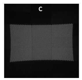
Dot projector '**C**' has a FOI of 70° x 40°, record efficiency above 70%, and dotuniformity-error <10%, making it an ideal platform for most 3D sensing applications where low power consumption is critical.
